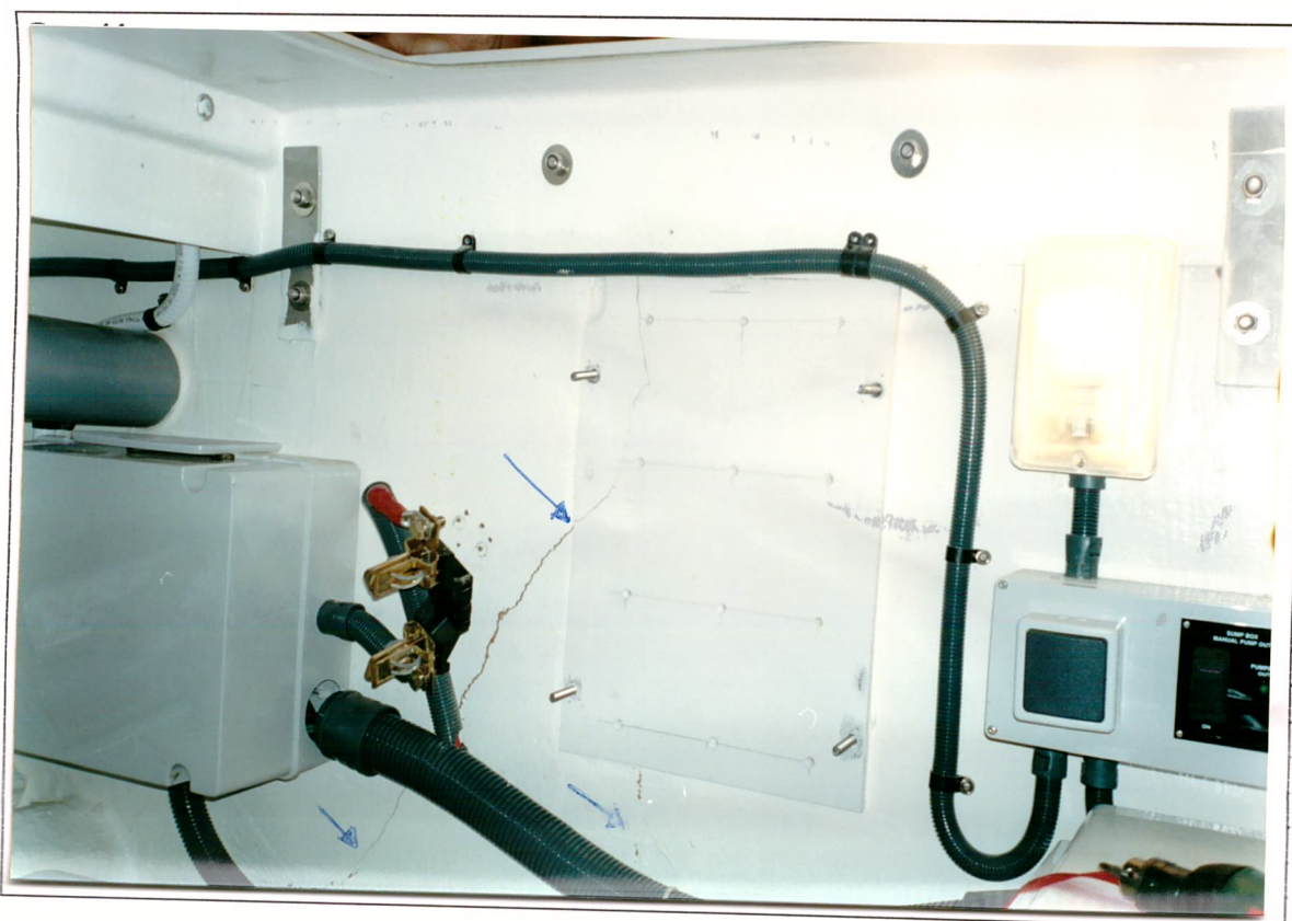
Antepara de ré no compartimento do thruster - Rachaduras diversas. Back bulkhead inside thruster compartment- Cracks.
