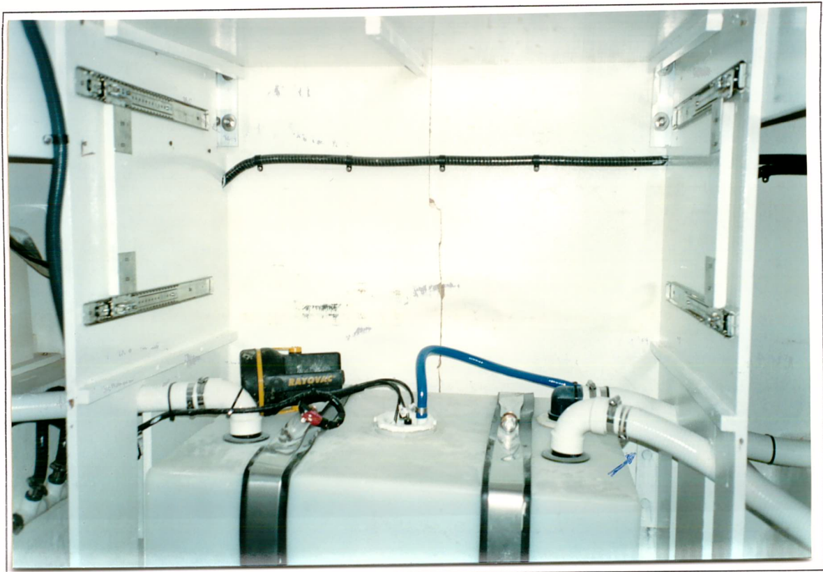
Compartimento da fossa - Rachaduras horizontais e verticais na antepara. Holding Tank compartment - Verticals and horizontal cracks in the bulkhead.
