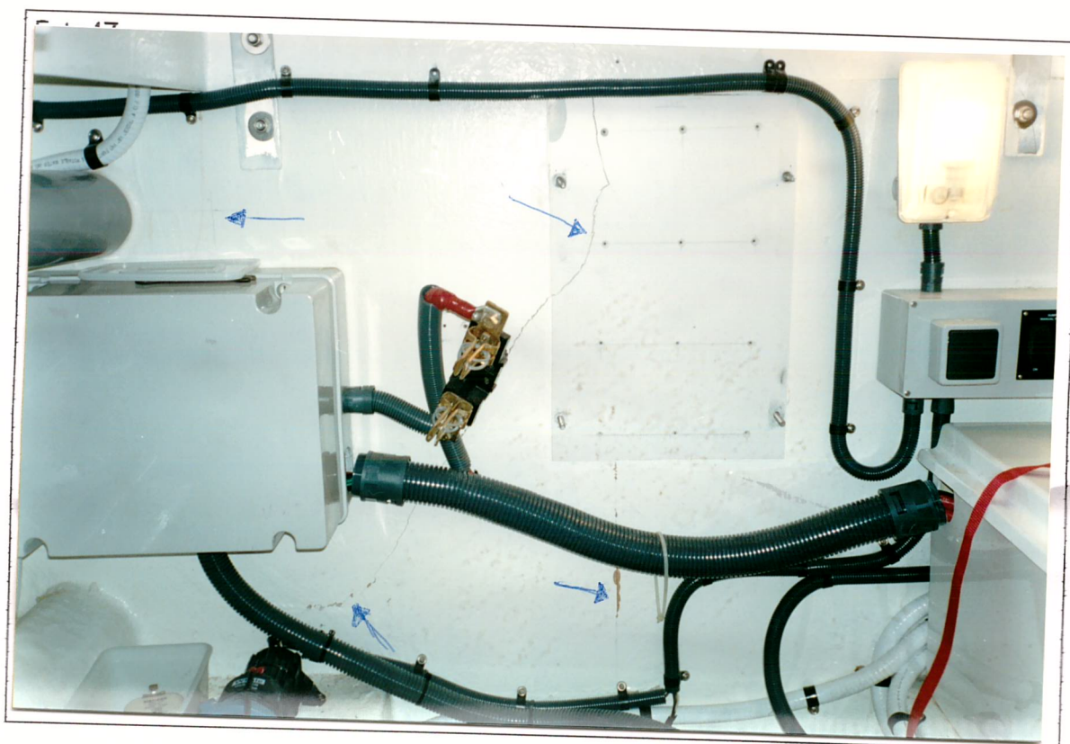
Antepara de ré no compartimento do thruster - Rachaduras diversas. Back bulkhead inside thruster compartment- Cracks.
