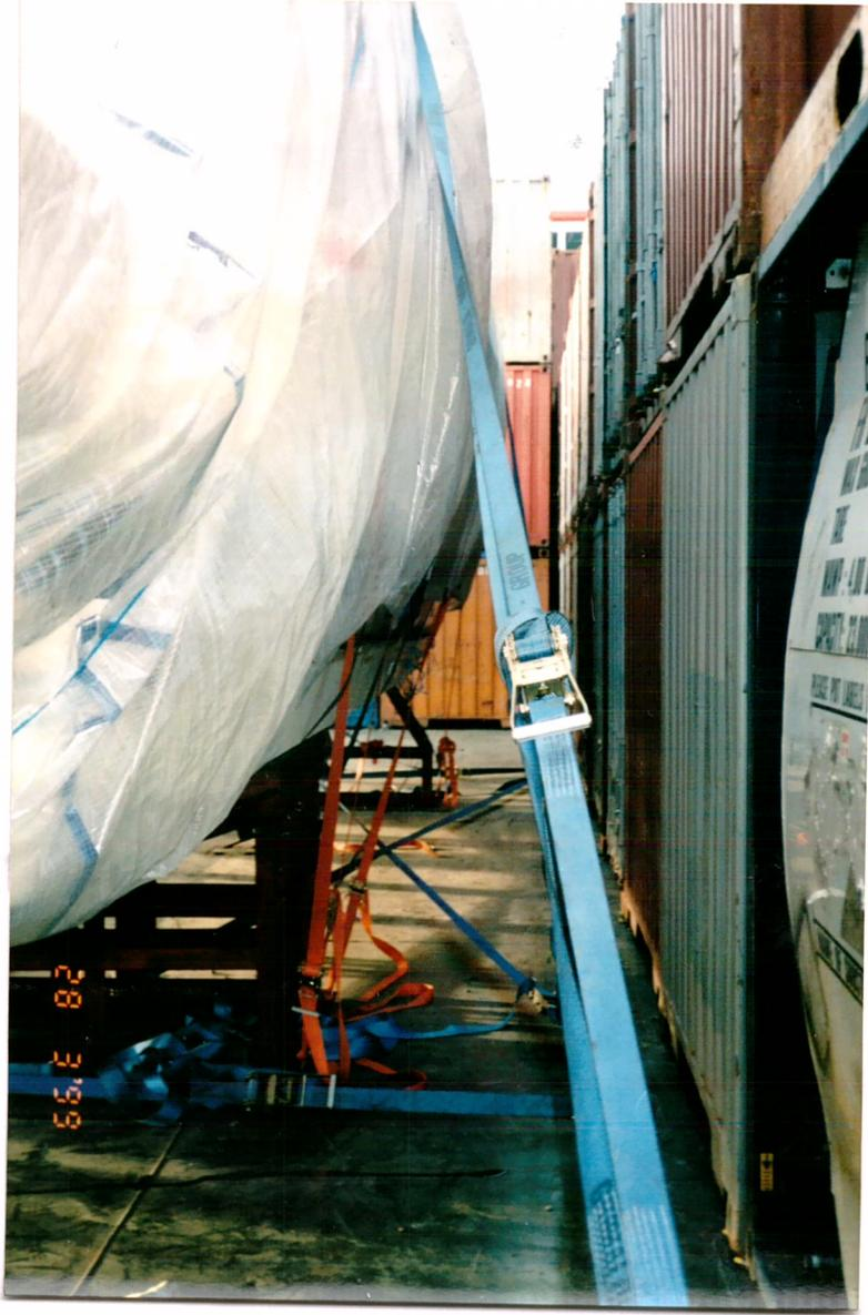
BOAT & CRADLE ALL SECURED IN BOARD & TIMBER UNDER HULL
